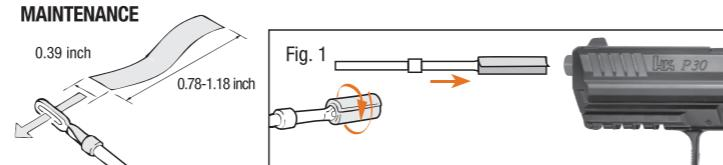
**EN** Perform routine inspections and maintenance to maintain proper operation. Put the safety "ON SAFE", remove the magazine. Prepare a thin rod with a length of 50 cm (not included). Attach a piece of cotton fabric to its end and clean the barrel with some silicone oil (Fig. 1).
