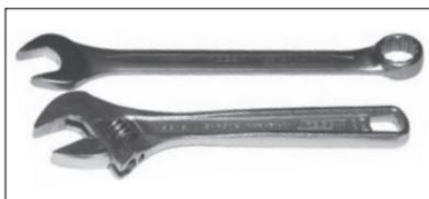
**STEP 1:** Installing a connector requires two wrenches - one for the hose and a second for the fitting. The wrench size for the hose is 14 mm. The wrench size for the fitting depends on the fitting.
