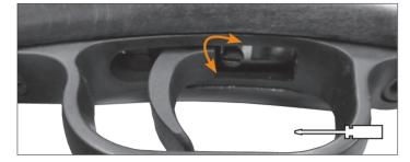
Turning clockwise decreases trigger travel Turning counter clockwise increases trigger travel.
